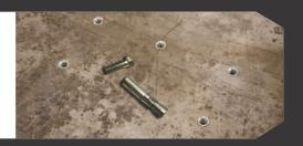
**ANCHOR BOLTS:** Internally threaded recessed drop-in anchors with caps install in your concrete floor and remain there permanently. The specially engineered anchors work by expanding against the sides of the hole and gripping the concrete. The holding power of each anchor bolt exceeds 14,000 pounds when properly installed.
