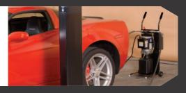
**PORTABLE POWER-UNIT:** Position the mobile power-unit cart at the front or rear of the vehicle. An optional power unit station kit with integrated lift controls and spring rewind hose reels is also available. Hydraulic lift controls can be located to best suit your needs and provide a central location for safe and easy operation.
