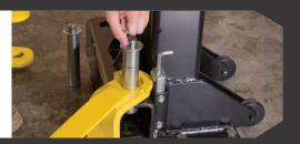
**COLUMNS & ARMS:** Roll the columns into position over the recessed anchors then secure each column to the floor using the five high- strength anchor bolts. Attach the adjustable lift arms to the MaxJax columns and install the quick drop-in pivot pins.
